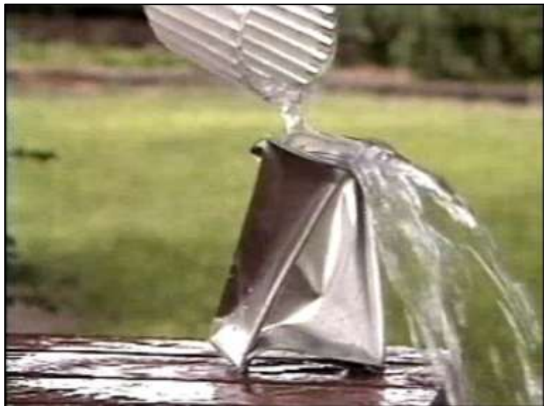
Figure 4: Contraction of Steam in Gallon Can
